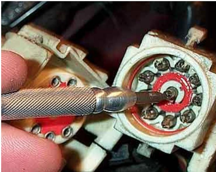
Before reassembly take some spray electrical contact cleaner and clean the male and female connectors. This problem is not isolated to the salt and pepper 10-pin connectors. The EGR sensor has a history of this problem, and many other Ford connectors. This is a regular maintenance repair you should plan on doing to your aging high mileage Ford.
