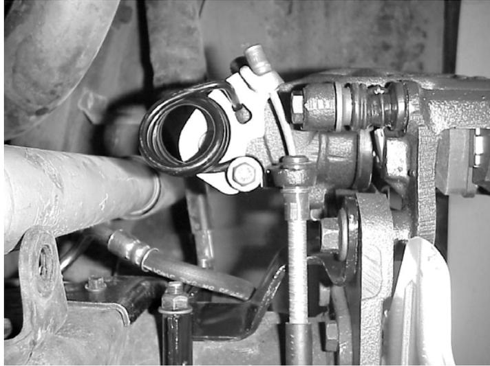
**STEP 2:** If your vehicle is a 1993 Mustang, install the rear brake cables (Item 52). Secure the cables to the body with the original clips.
