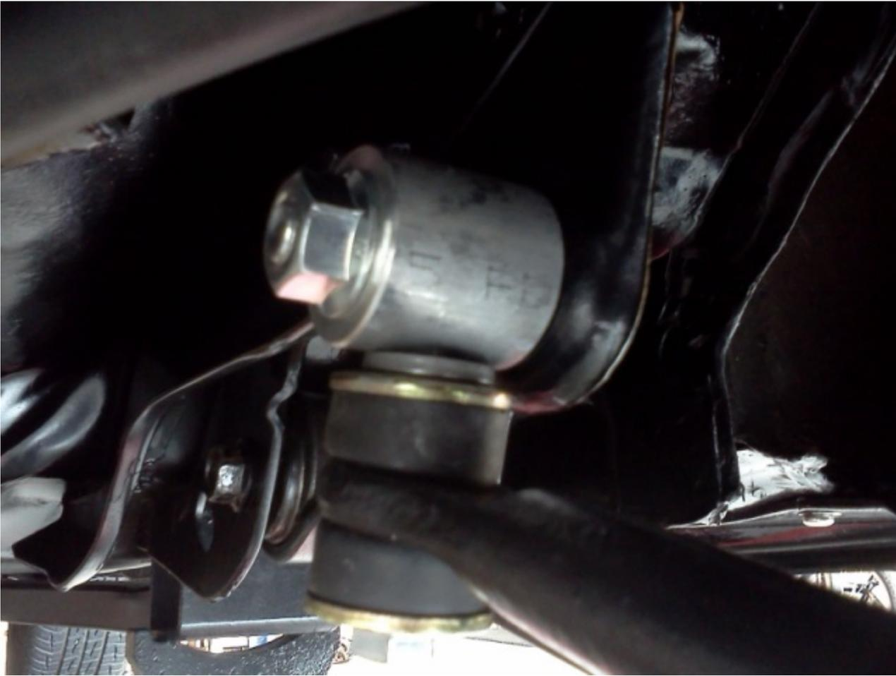
\*I added an extra 3/8" washer between the aluminum connector and the top cupped washer so the bushings would compress properly. In the future I will probably use a 3/8-16x2" bolt and get rid of the extra washer.
