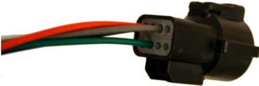
If you have an 89-90 Mustang 5.0 MANUAL TRANS OXYGEN SENSOR HARNESS, it should be pinned like this. Be sure to pin your new harness like this:
