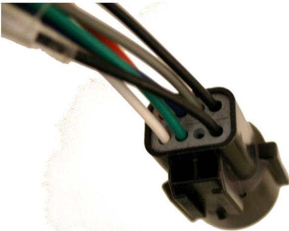
If you have an 91-93 Mustang 5.0 MANUAL TRANS OXYGEN SENSOR HARNESS, it should be pinned like this. Be sure to pin your new harness like this:
