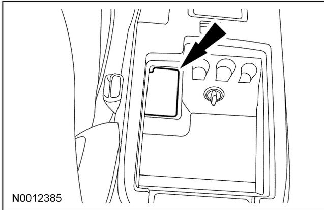
2. Position the parking brake handle up at the fourth notch to access the adjuster nut.
