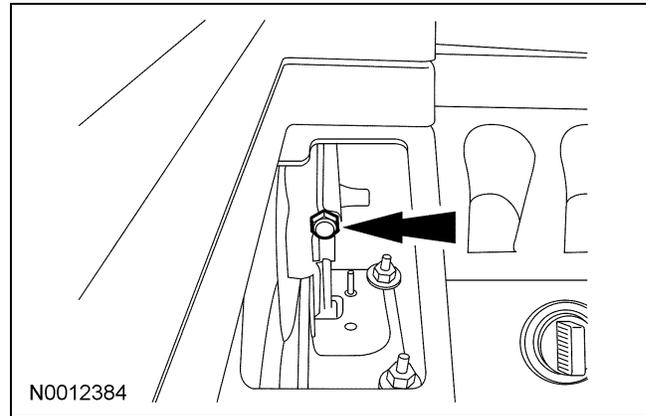
4. Apply the tension by tightening the parking brake cable adjustment nut until there is no lash in the system with the handle in the lowered position.
